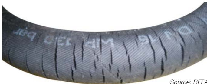
Figure 6: A hose with a cracked outer cover due to being exposed to heat 20° C higher than its maximum working
