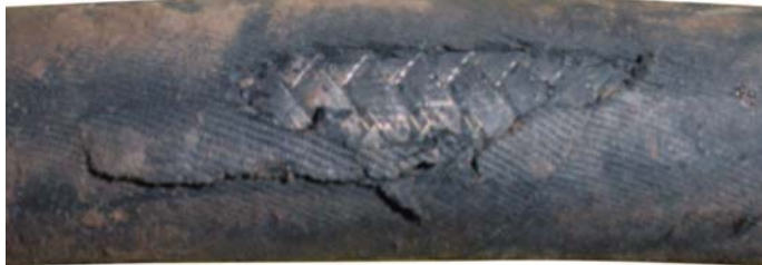
Figure 7: Hydraulic hose with its protective cover removed by abrasion
